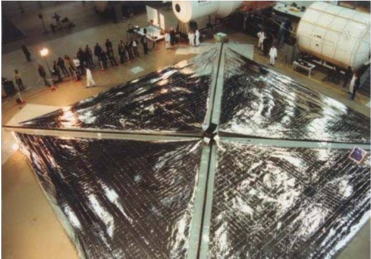
Figure 1 – Ground deployment test of a (20 m) 2 sail at DLR Cologne, 1999
