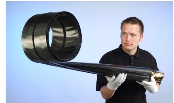
Deployed De-Orbit Sail drag sail using DLRS CFRP boom technology
