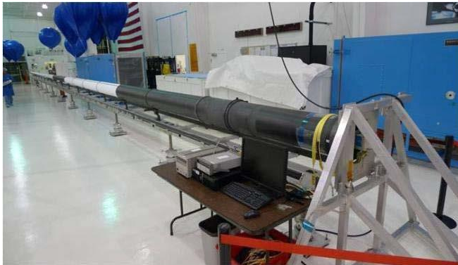
Telescopic composite mast deployed by an internal metal STEM boom (Courtesy of Northrop Grumman)
