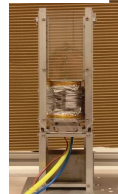
Inflatable Aluminum laminate boom of Inflatesail (Courtesy of University of Surrey)
