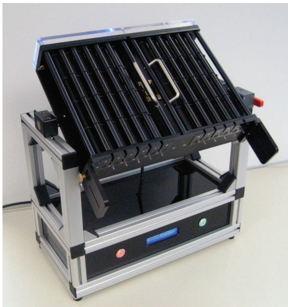
Figure 1. Cuvette clinostat provided by the German Aerospace Center (DLR).
