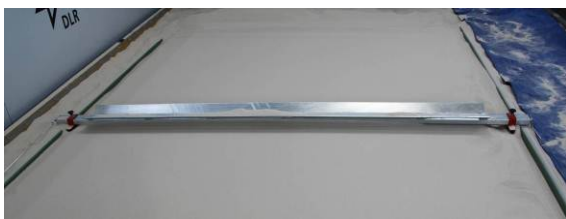
Fig. 5: Test bed for the drop tests
