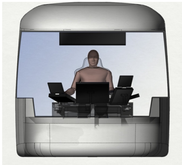
Figure 5. AIM Modular Mockup Rail including driver's cab
