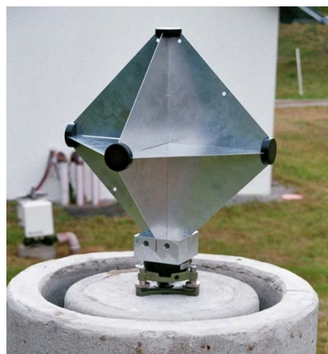
Figure 1: Octahedron reflector placed on a concrete pillar of the local geodetic survey network in Wettzell.
