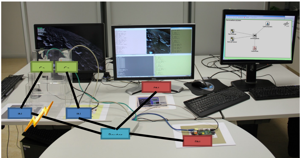
Figure 5-1 OBC-NG navigation camera setup
