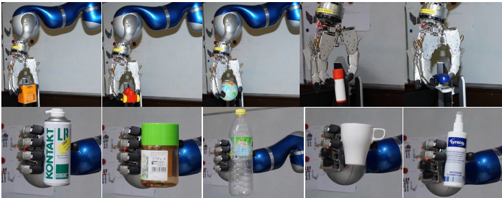
Fig. 6. Examples of successful grasps, from the side or above, of different objects with various object position errors.
