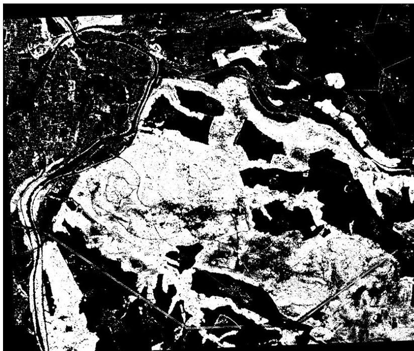
Figure 7.2: HySpex VNIR forest mask derived from LiDAR mask, NDVI mask and NDBRI mask
