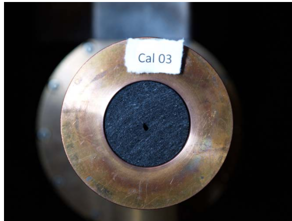
Figure 2: Probe with mounted CALCARB sample.
