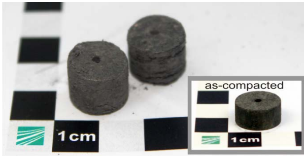
Fig6 Sample MHC-D before and after 1000 cycles
