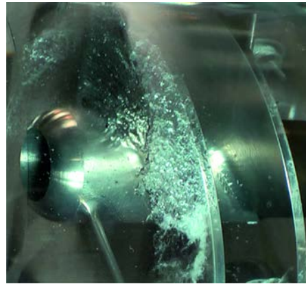
Figure 5 Cavitation at Inducer Inlet Source Technical University, Kaiserslautern
