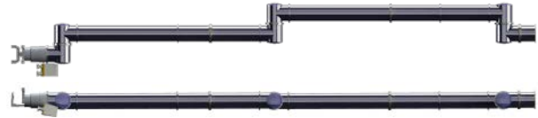
Figure 3: Robotic arm in zero (stretched) configuration with gripper and stereo camera system attached.
