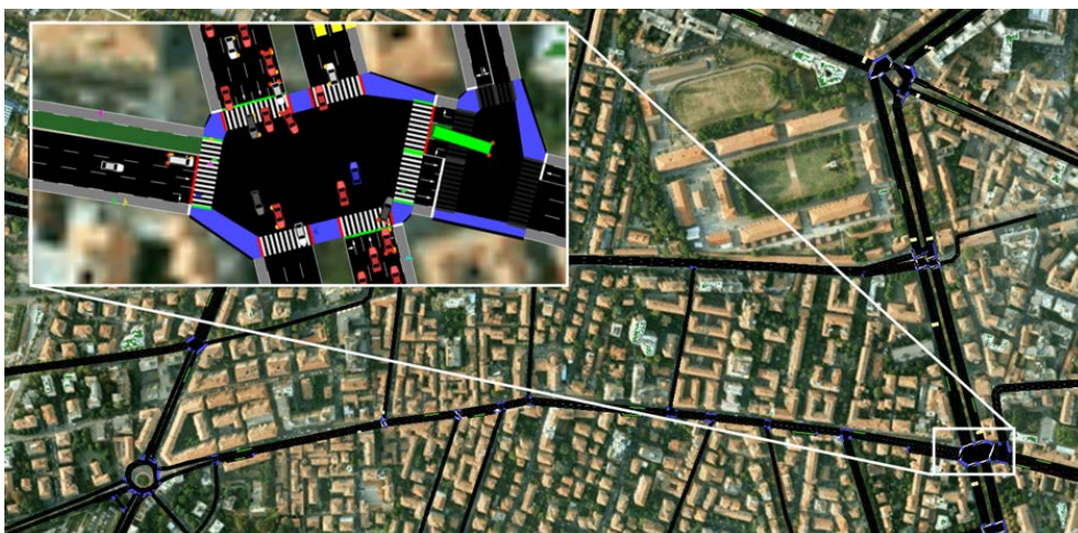
Figure 7 - The area around the “Andrea Costa” road in Bologna as simulated with pedestrians in SUMO
