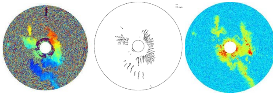
Figure 45: Wind field monitoring with PSR radar weather channel. Left: Doppler radial velocity in rain cloud. Centre: Wind field assessment based on Doppler information. Right: Atmospheric turbulence map based on high resolution Doppler processing.
