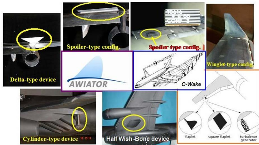
Figure 76: Illustration of wing add-on devices investigated in different EC projects.
