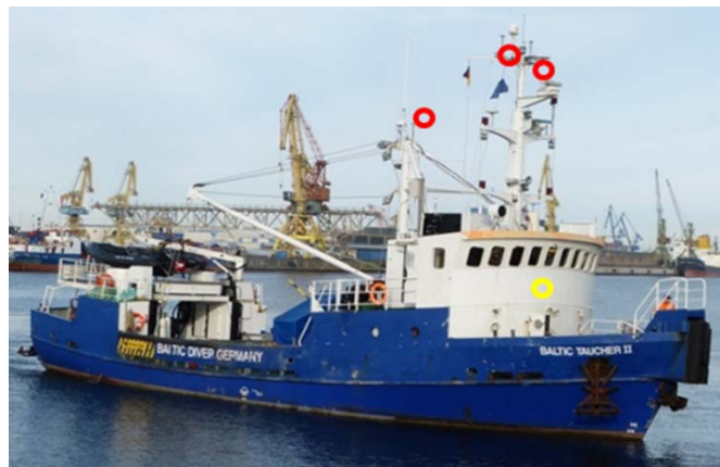
Figure 1. Baltic Taucher II test vessel. Yellow circle represents the IMU placement and the red circles stand for GNSS antenna positions (3x).
