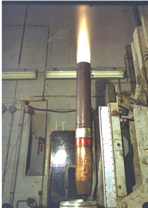
Figure 4. Exemplary propulsion test of a RAM-jet configuration in VMK.
