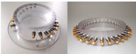
Fig. 6: Bubble trap (left) and sensor ring (right) equipped with piezoelectric transducers.
