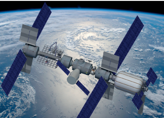
Figure 1: Illustration of DLR's Orbital-Hub concept during the docked phase for the servicing of the Free-Flyer consisting of an external science platform and a pressurized laboratory.
