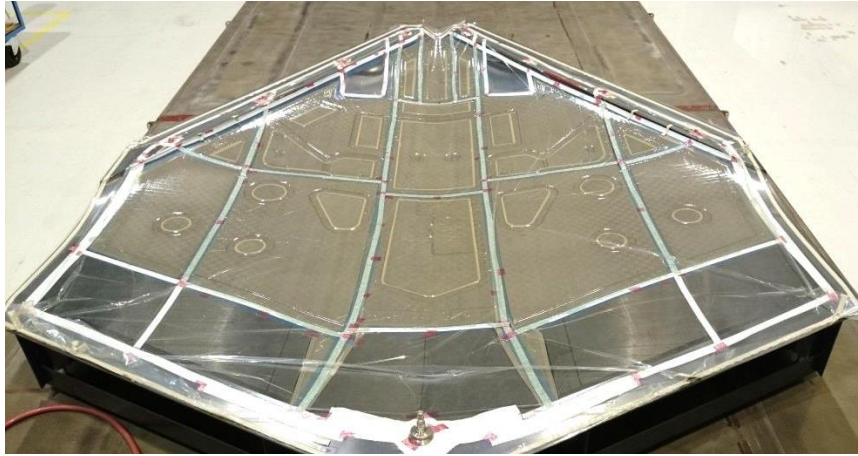
Figure 25: Sagitta lower skin in the CFRP tooling after the curing process, covered with the vacuum bagging.
