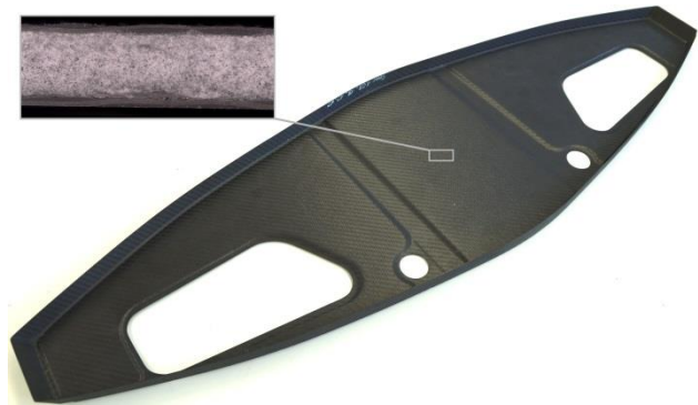
Figure 26: Spar 1 with cut-outs for the jet engine intakes, enlarged cross section of the sandwich area
