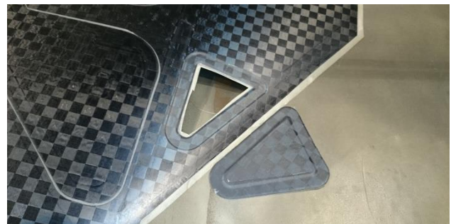
Figure 24: Integrally manufactured cover of the Sagitta lower skin
