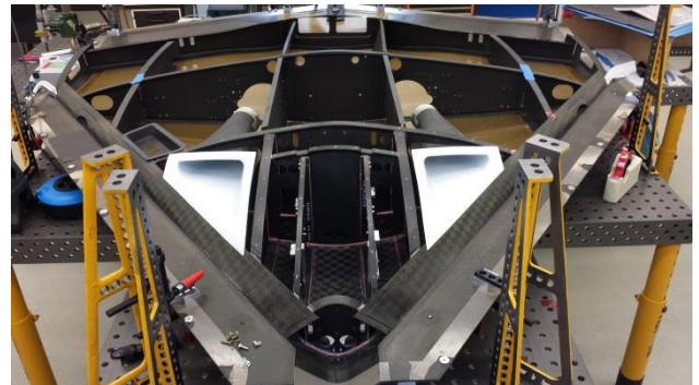
Figure 29: Assembly rig of the Sagitta demonstrator, preliminary fitting of the inner structure with the upper shell
