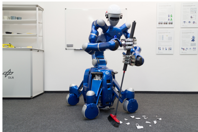
Fig. 1. The humanoid Rollin' Justin sweeping shards of a broken mug as example for a compliant manipulation task.
