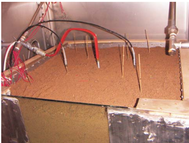
Fig. 1 Thermal probes used for determining heat conductivity and temperature profiles. In the center, one EXTASE probe is visible, to the left and to the right of it the Hukseflux TP02 sensors are inserted into the soil. The wooden rods mark the positions of the RTD sensors, which are mounted vertically along the rods with about 5 cm mutual distance
