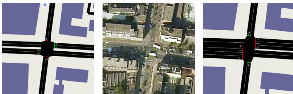
Figure 3.15: Adaptations to the OSM network; left: original OSM data, centre: Google Earth image; right: network after adaptation (from: DRIVE C2X Deliverable D22.1 “Methodology Framework available”)
