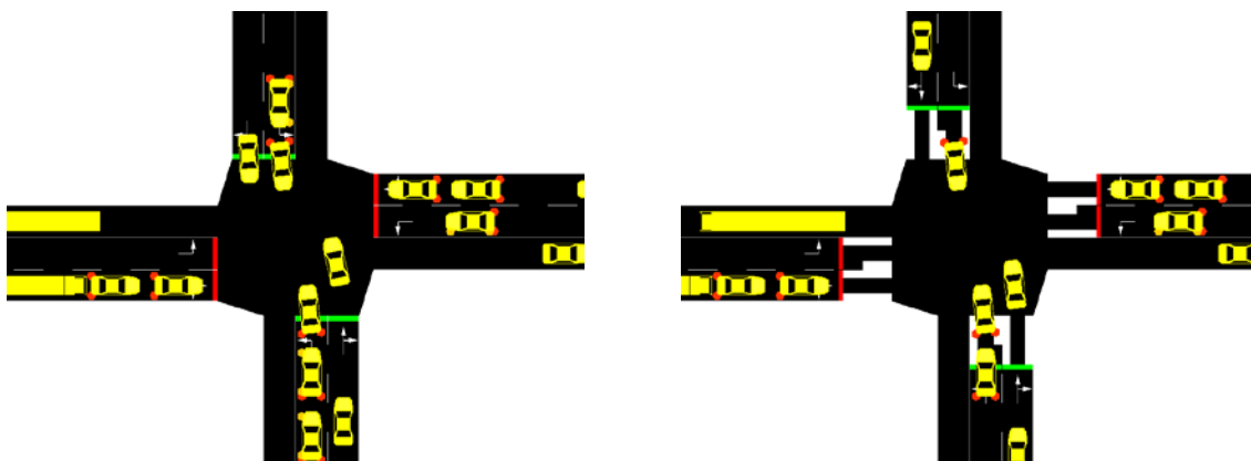
Figure 5.1: The same intersection, once not regarding pedestrian crossing areas (left) and once with halting lines that regard the area of pedestrian crossings (right)
