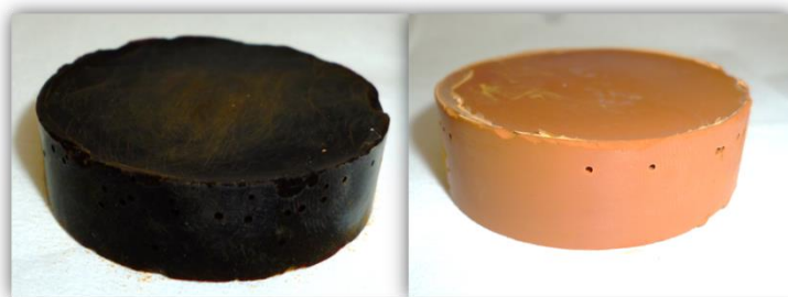
Fig. 1. Representative RF aerogels prepared at pH 7 (left) and pH 6.5 (right), respectively.
