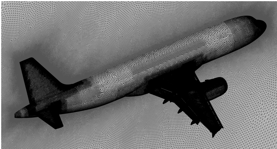
Figure 3. A320-232 CFD surface (black) and symmetry plane (gray) meshes.
