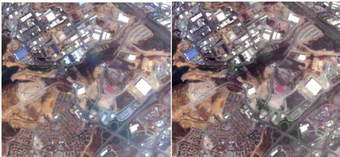
Figure 13: Subset of a RapidEye scene before (left) and after atmospheric correction (right).
