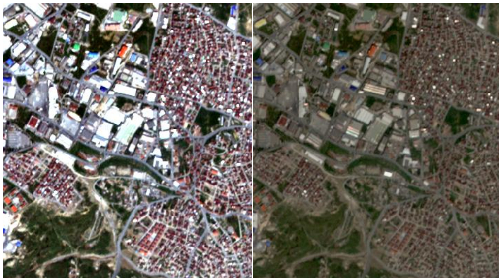
Figure 14: Snippet of an atmospheric corrected RapidEye scene before (left) and after histogram stretching (right).
