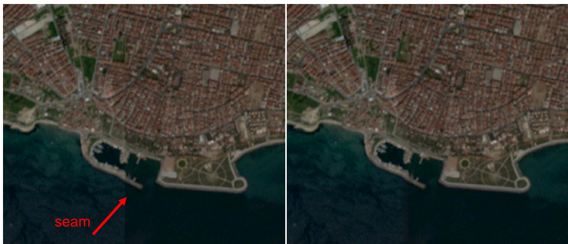
Figure 15: Subset of the mosaic with blended and blurred (feathering) seam (right) and without (left).
