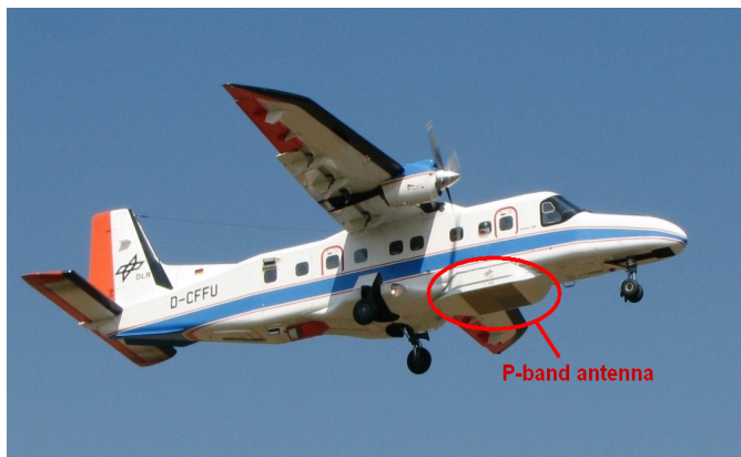
Fig. 1. The P-band antenna mounted under the aircraft Do-228.
