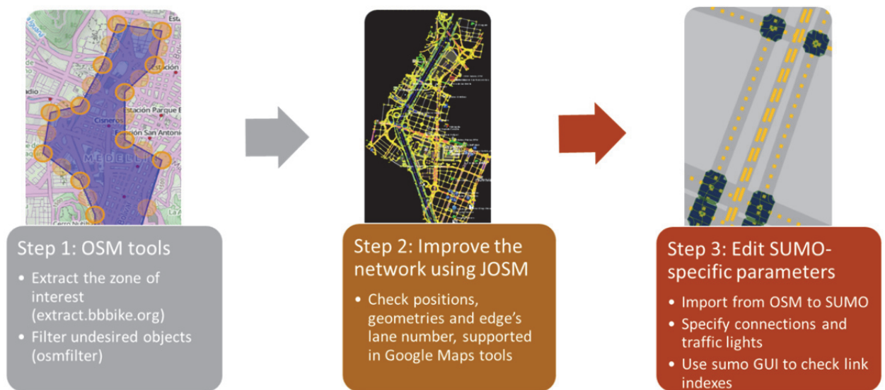
Figure 3-1: A general methodology for creating simulation scenarios for SUMO, using information from Open Street Maps (OSM).
