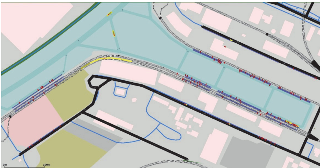
Figure 8-15. The harbor of Brunswick in the SUMO-simulation; containers are displayed in red, vehicles in yellow and container stops in blue
