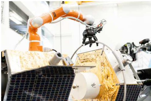
Fig. 8: The servicer manipulator is about to grasp the client satellite
