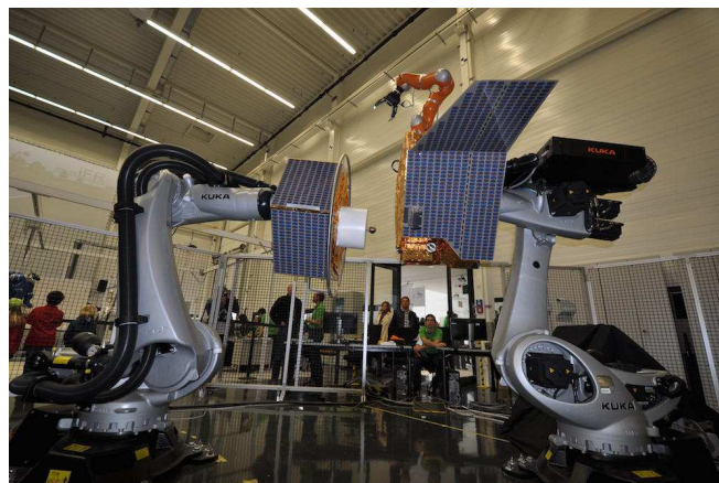
Fig. 1: Overview of the OOS-SIM. Left: Client satellite; Right: Servicer satellite and manipulator
