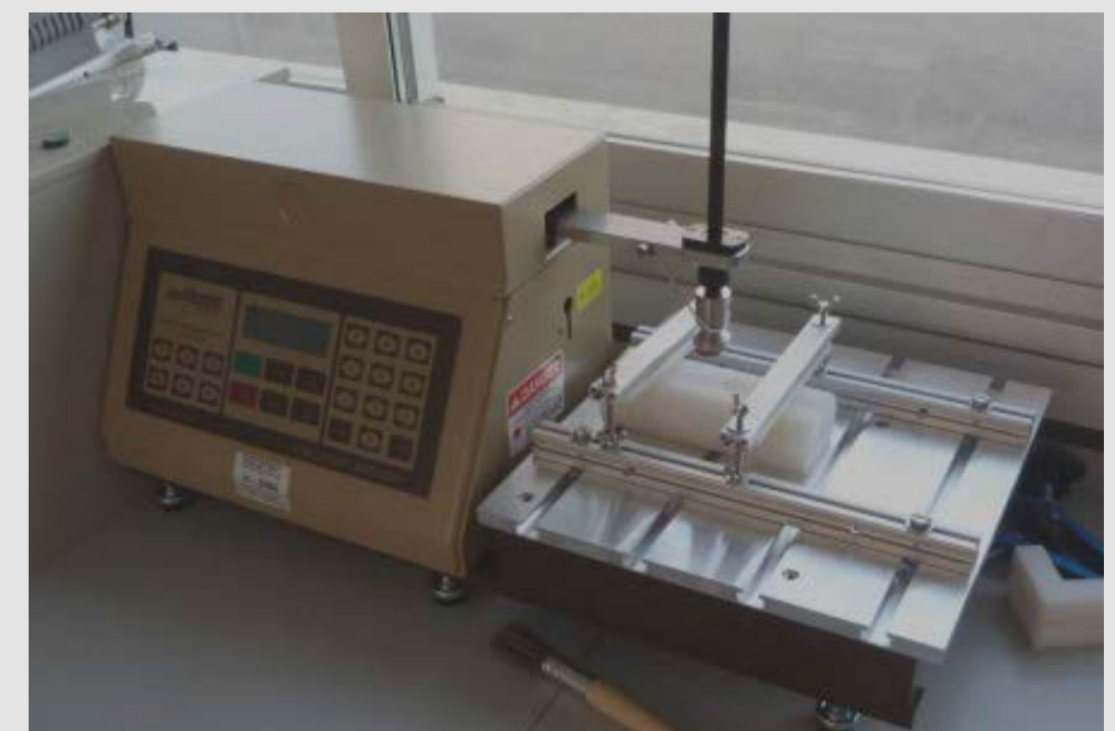
Figure 6: Taber Linear Abrasion Test for AR-coating testing
