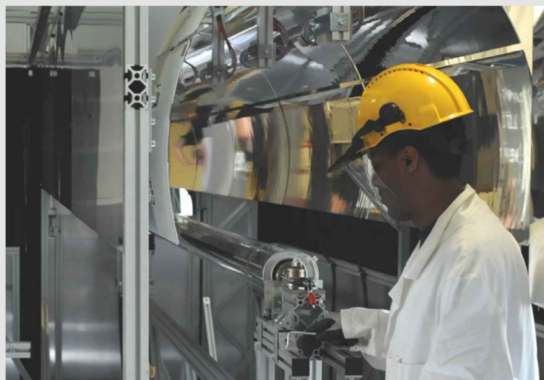
Figure 2: Linear focus solar simulator
