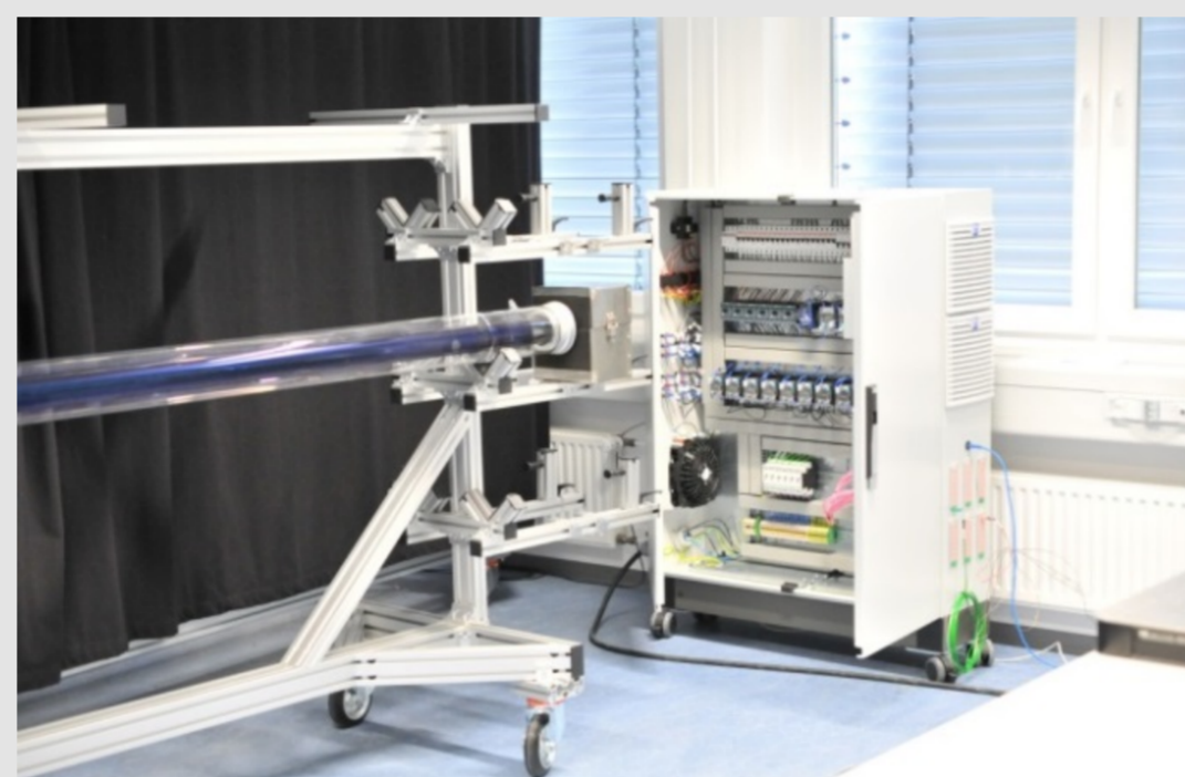
Figure 4: Test bench for overheating and thermal cycling of parabolic trough receivers
