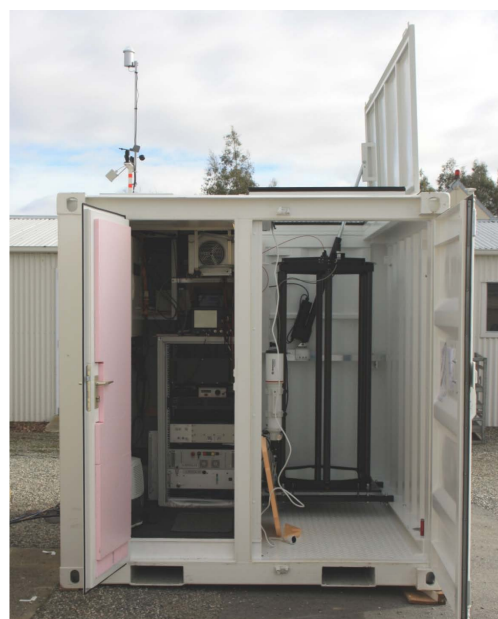
Fig. 2: Container with laser and receiver system (left) and telescope (right)
