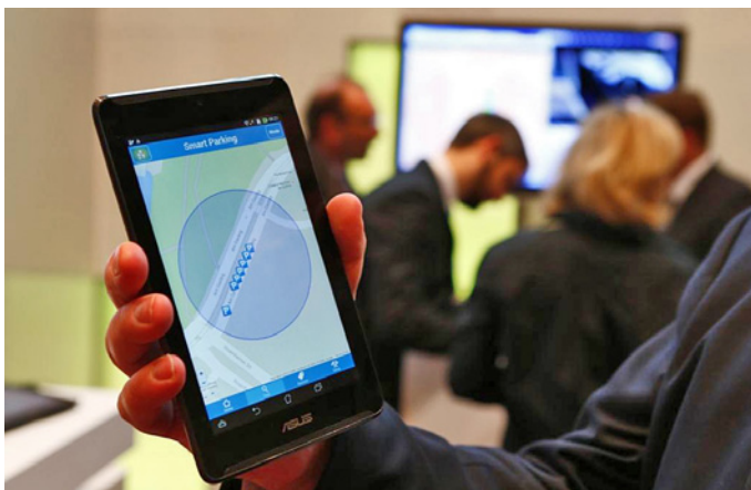
Figure 3: The parking control center distributes the occupation status to road users via smart phones, tablets or navigation systems.
