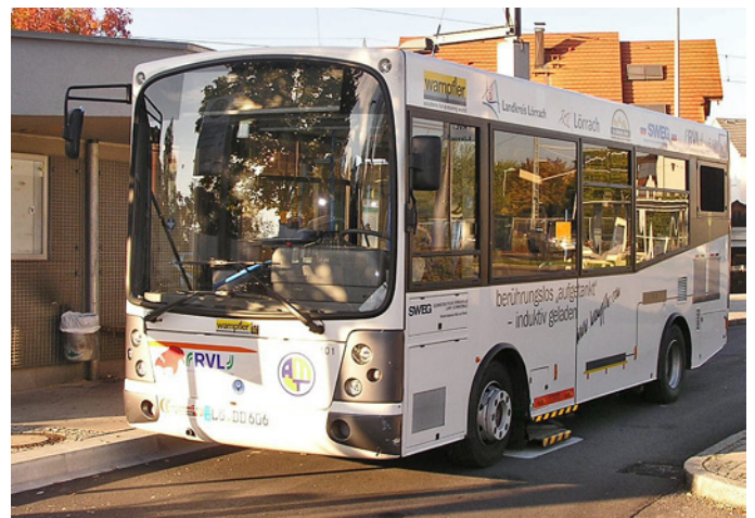
Figure 1: Contact-free recharging e-bus. All photos: City of Lörrach
