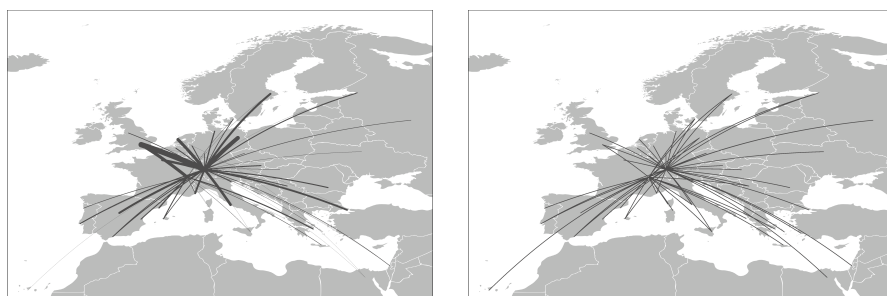
Fig. 3. (a) demand network of selected airline net, width of connection indicates amount of demand; (b) network of potential flights.
