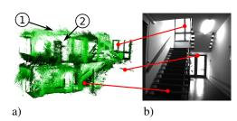
Figure 1: a) The acquired 3D samples shown as a point cloud. b) The scanned staircase as a photograph.
