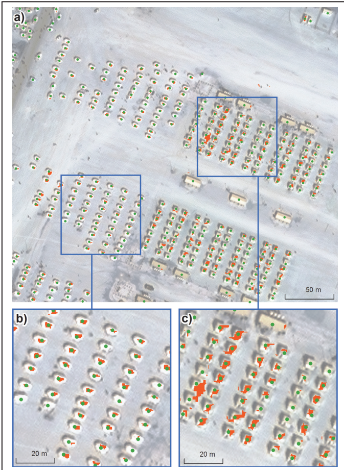
Fig. 2. Superimposition of visually/manually digitized (green dots) and semi-automatically derived (red polygons) shelter locations, based on the Al Zaatari data set of WorldView-2, as of January 03, 2013. For the semi-automatic mapping a sample supervised approach was used. Part a) showing test zone of the Al Zaatari Scene. Part b) and c) showing zoom-windows with slightly different results in segmentation characteristics.
