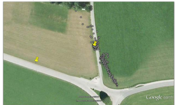
b) weaker repeater signals, attenuation of 10 dB
