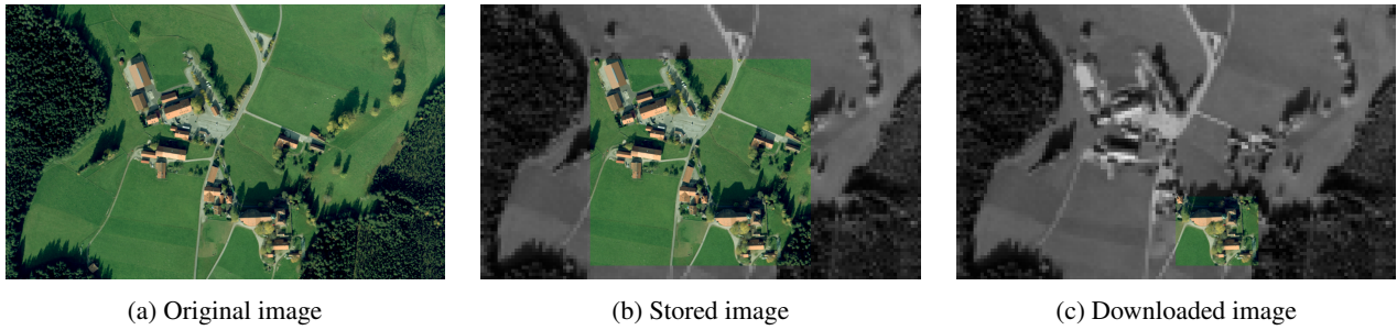
Fig. 2: The same image at three different stages: a) before compression, b) after compression and c) as it is requested by the ground station.
