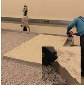
Figure 5.3: Scanning of terrain model, laser tracker in background. close-up shows scanner and red laser pattern
