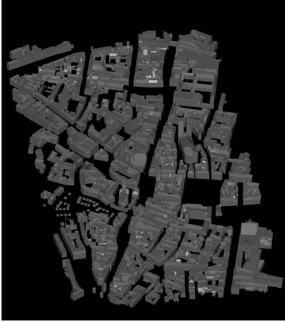
Figure 7: Rendered image of CityGML model, representing the line-of-sight of the virtual SAR sensor.
