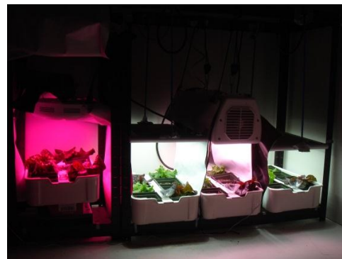
Fig. 4: Lamp set-up in the sciences lab. Left to right: red and blue UFO LED lamp, KSC white panel, Heliospectra LX 60, and KSC white panel.
