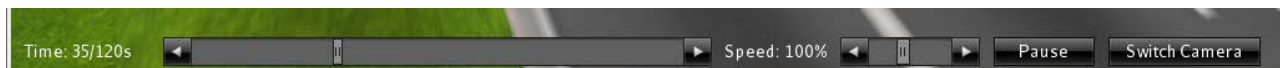
Figure 8-3: Controls for the visualization: the current time (shown on extreme left) can be freely selected using the slider on the left. Speed can be altered using the speed slider. The simulation can be paused at any time using the pause button, and the pre-defined camera positions can be used by clicking "Switch Camera".
