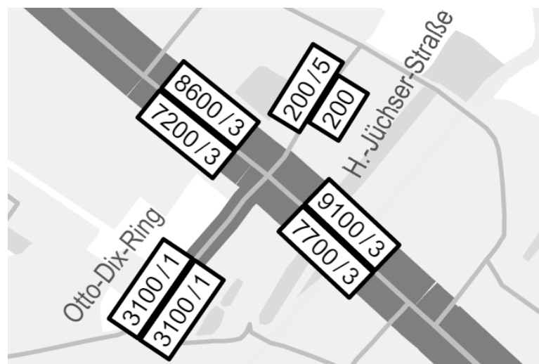
Figure 6-1: Part of a traffic volume map (format: daily traffic / percentage of heavy traffic)
