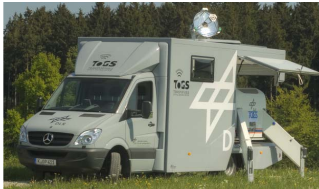
Figure 11: Transportable optical ground Station (TOGS)
