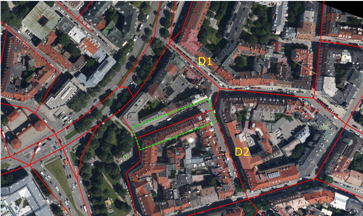
Figure 5.1: Accuracy of roads from the Navteq database in the center of Munich. The database is from the year 2008. It can be seen what problems are posed when it is aimed to only extract the road surface. The dashed green rectangle shows an extreme case of inaccuracy (All other roads must be extracted using the same buffer size as the most inaccurate one.). The normal application is routing and therefore the shown accuracy is good enough. Additionally, the yellow D1 and D2 indicate the roads of Datasets 1 and 2, respectively.
