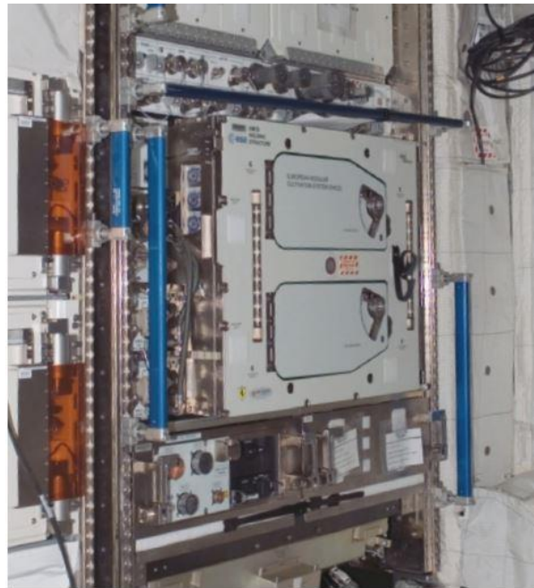
Figure 8. EMCS in EXPRESS Rack-3 inside ESA Columbus Module (since April 2008) 47 .
