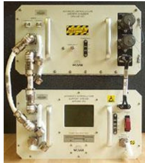
Figure 5. Advanced Astroculture ISS plant growth chamber 34 .
