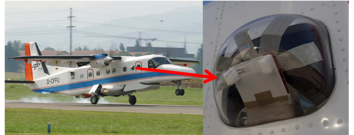
Fig. 2. DLR's DO 228-212 research aircraft (left) and right observation window with installed LTE FRITZ!Box modem (right).
