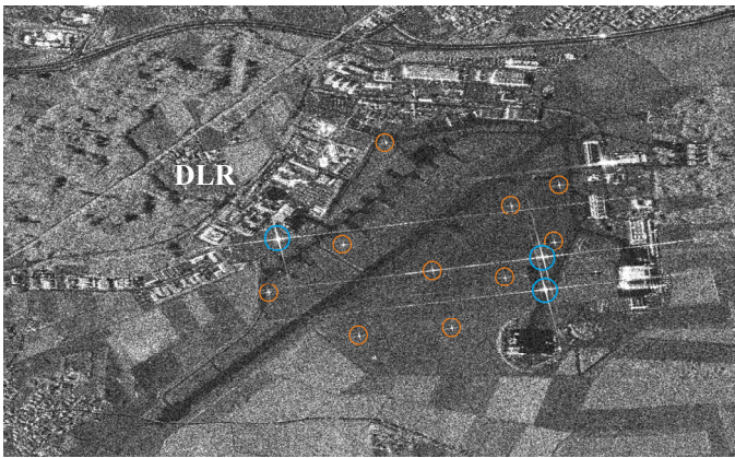
Fig. 4. One of seven RADARSAT-2 images of three transponders with strong backscattering and ten 1.5 m corner reflectors at Oberpfaffenhofen, Germany, acquired in February 2014.
