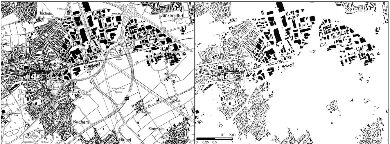
Fig. 3. Extraction of building footprints from DTK-25. The left part of the figure displays the black layer of the digital topographic map 1:25 000 (DTK-25) with the map content including buildings, streets, railways, and lettering. After application of the building extraction procedure, only building footprints remain (right part of the figure). These extracted building footprints are further used for the generation of the building block models in combination with the Cartosat-1 DSM. Topographic map: GeoBasis-DE/BKG (2010).
