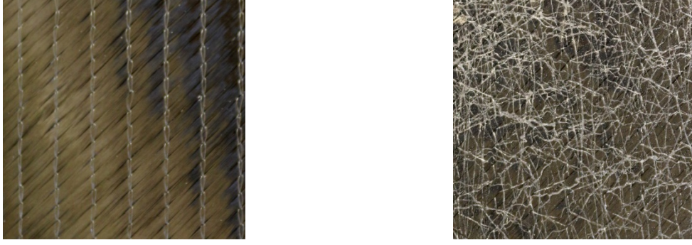
Figure 12: Samples of NCF weft side (left) and warp side with toughener (right)
