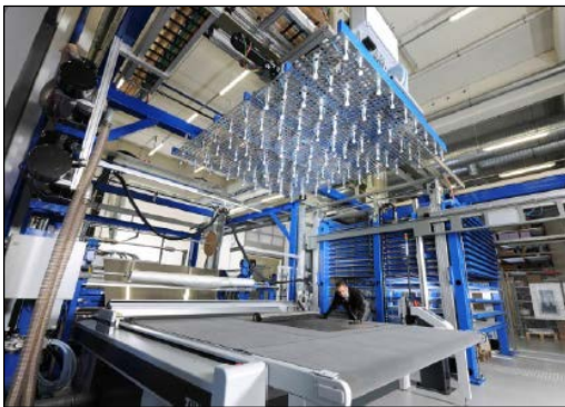
a) CNC cutter and ply handling portal robot
