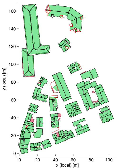
(c) Green areas: True positive estimated segments TP_e ; red areas: False positive estimated segments FP ; black polygons: true positive (detected) reference segments TP_r ; red polygons: false negative (missed) reference segments FN
