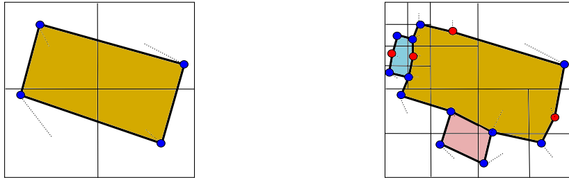
(a) Rectilinear flat segment represented by four hyperpoints (blue points), in a maximally collapsed quadtree; quadtree cells plotted with black lines; dotted lines indicate the centers of the quadtree cells from which the hyperpoints are computed (b) Additional adjacent rectilinear segments represented by more hyperpoints. The quadtree cannot collapse, because the additional hyperpoints have to be created, such that also unnecessary hyperpoints are created for the other cells of the non-collapsed quad (red points); dotted lines indicate the centers of the quadtree cells from which the hyperpoints are computed
